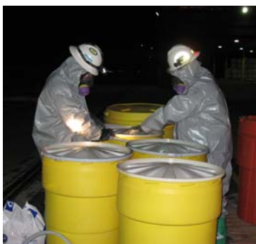
HEPACO personnel overpacking damaged containers.
